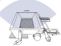
Release the lock. Then open the slide gate by rotating the operating shaft with a lever. The position of the slide gate will determine the rate of discharge. Open completely for maximum flow.
