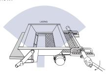
After discharge is complete, close and lock the slide gate, then close and lock the sanitary shield. Close the hatch.
